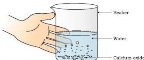
Figure 1.3 Formation of slaked lime by the reaction of calcium oxide with water
