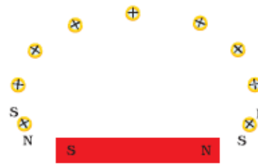
Figure 13.3 Drawing a magnetic field line with the help of a compass needle
